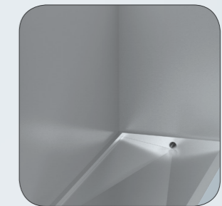
Material thickness of stainless steel drain pan \geq 1.5 mm Slope design \geq 3\%
